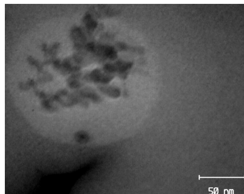
Figure 10. TEM image of complex PAA / PEO in the presence of 10% \beta CD.
