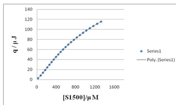
**Figure 1.** Comparison between the experimental heats,  $q$ , ( $\Upsilon$ ), for S1500+lysozyme interactions and calculated data (lines) via Eq. 1.
