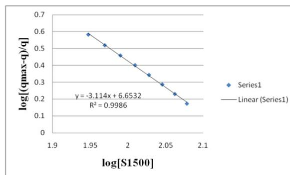
**Figure 3.** The fitting of heats of S1500+lysozyme interactions for the second set of binding series (in the high concentration of S1500).
