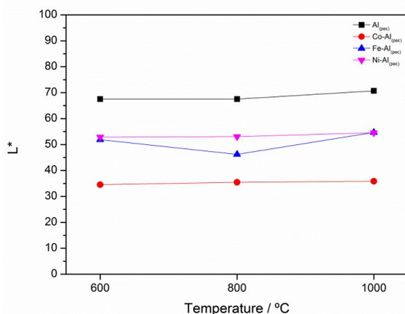
**Figure 1.** Graphs of luminosity intensity ( $L^*$ ) as a function of temperature and pigment group.
