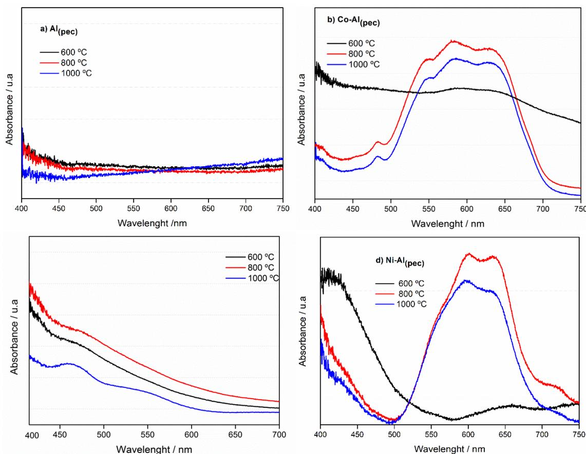
**Figure 5.** Electronic spectra of the a) Al(pec), b) Co-Al(pec), c) Fe-Al(pec), and d) Ni-Al(pec) pigments, prepared upon heat treatment at 600, 800 and 1000 °C, in the visible range.
