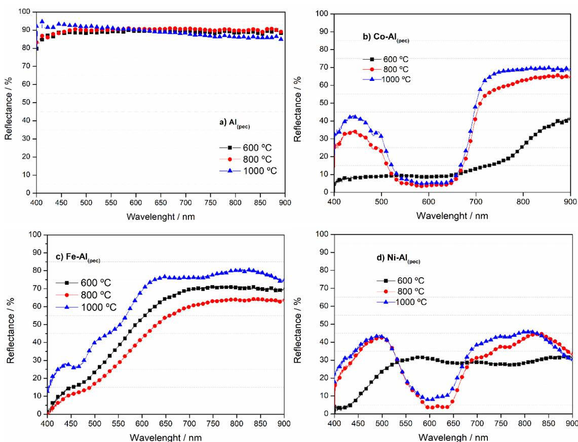
**Figure 4.** Diffuse reflectance spectra (VIS-NIR) of pigments: a)  $\text{Al}_{(\text{pec})}$ ; b)  $\text{Co-Al}_{(\text{pec})}$ ; c)  $\text{Fe-Al}_{(\text{pec})}$ ; and d)  $\text{Ni-Al}_{(\text{pec})}$ .
