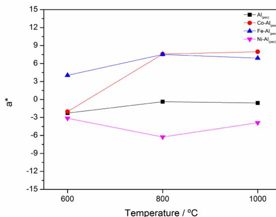
**Figure 2.** Graphs of the red-green color intensity parameter  $a^*$  as a function of temperature and pigment group.
