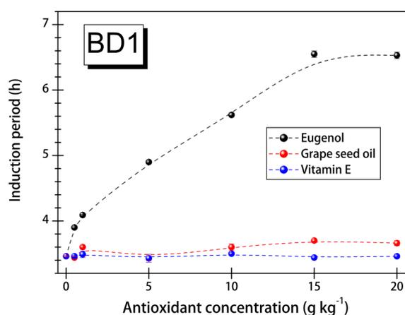
**Figure 1.** Induction period behaviors for waste cooking oil derived biodiesel (BD1) as a function of the type of antioxidant and the additive concentration.
