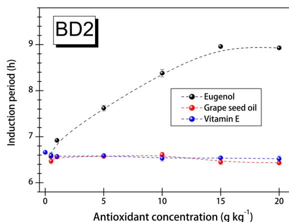
**Figure 2.** Induction period behaviors for animal-vegetable blend derived biodiesel (BD2) as a function of the type of antioxidant and the additive concentration.
