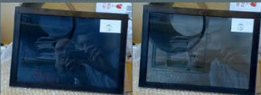
SPD smart window in dark (left) and clear (right) states with 0 and 100 V peak applied.
