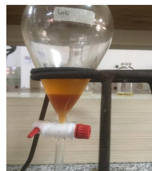
Fig. 5 Final Transesterification of Waste Cooking Oil with SrO-KF Catalyst in Separation Funnel.
