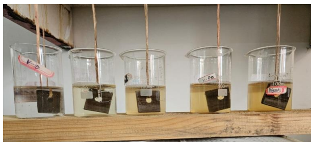
Fig. 11. Weight loss method for blank, 10 mg, 20 mg, 30 mg, 40 mg of FeO-NPs.
