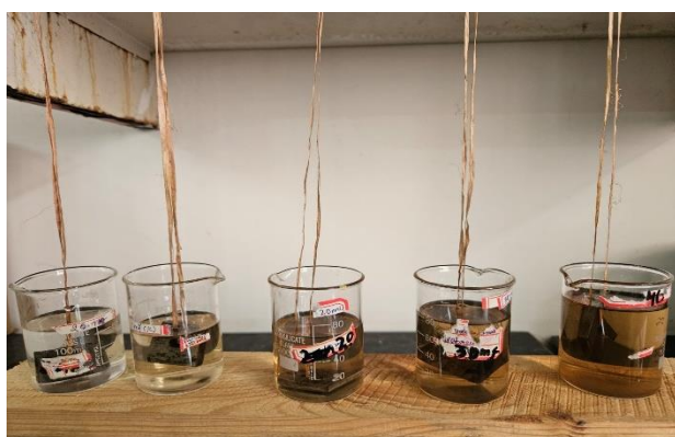
Fig. 14. Weight Loss for blank, 10 mL, 20 mL, 30 mL and 40 mL.
